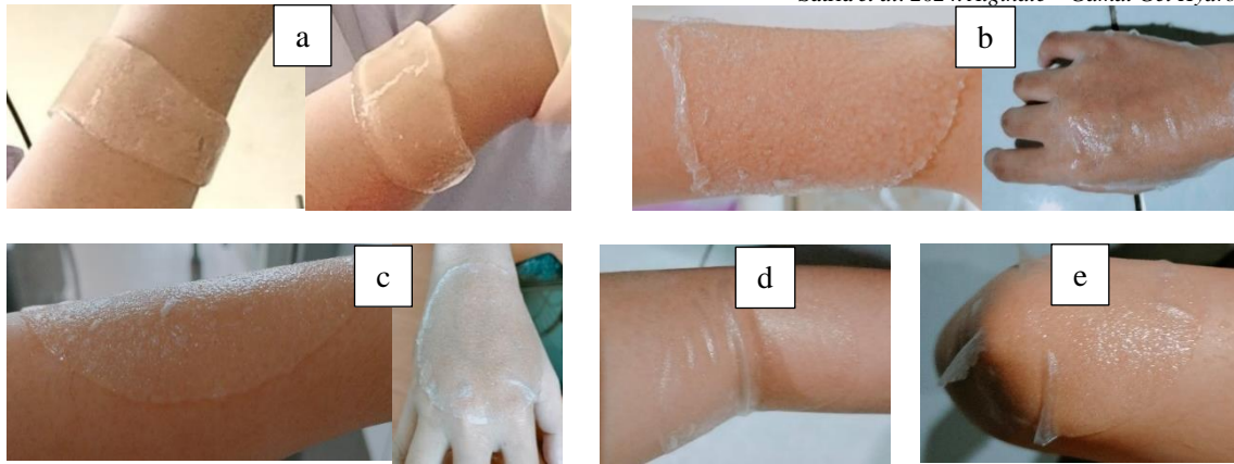
Figure 6. General elasticity of hydrogel films of (a) 1% w/v, (b) 3% w/v, (c) 5% w/v alginate concentration, (d) on the crook of elbow, and (e) on elbow
